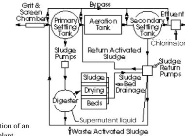
**Figure 1**. Illustration of an activated sludge plant
