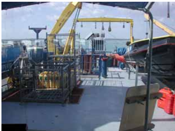
This is a CTD sampler - conductivity (for salinity), temperature, depth. These samplers have been used for a long time by oceanographers and biologists alike, to find out the conditions at different depths of the oceans. In the background you can see the sampling bottles that can be computer-controlled to open and take a sample at pre-set depths.
