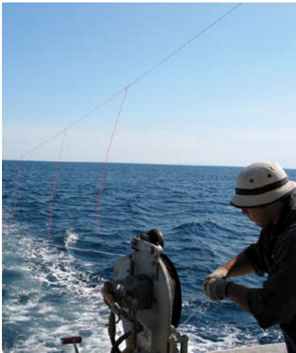
The bird-scaring line and streamers set off the back of the longline vessel, above where the hooks are being put in the water. These make it harder for the birds to get to the baited hooks. (Dave Cranston, courtesy AFMA)
