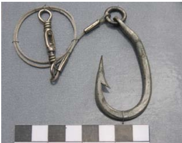
A longline hook with wire leader, the wire makes it harder for an animal, such as a shark to bite through the line if caught. Wire leaders are banned in some Australian fisheries to reduce the bycatch of sharks. (courtesy BRS)
