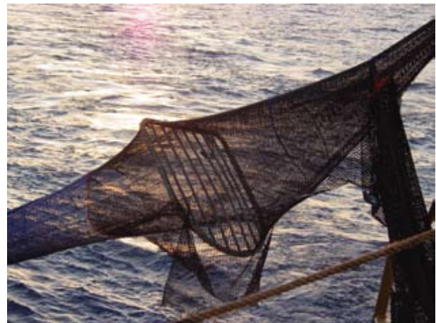
A Turtle Excluder Device in a prawn trawl net. (courtesy AFMA)
